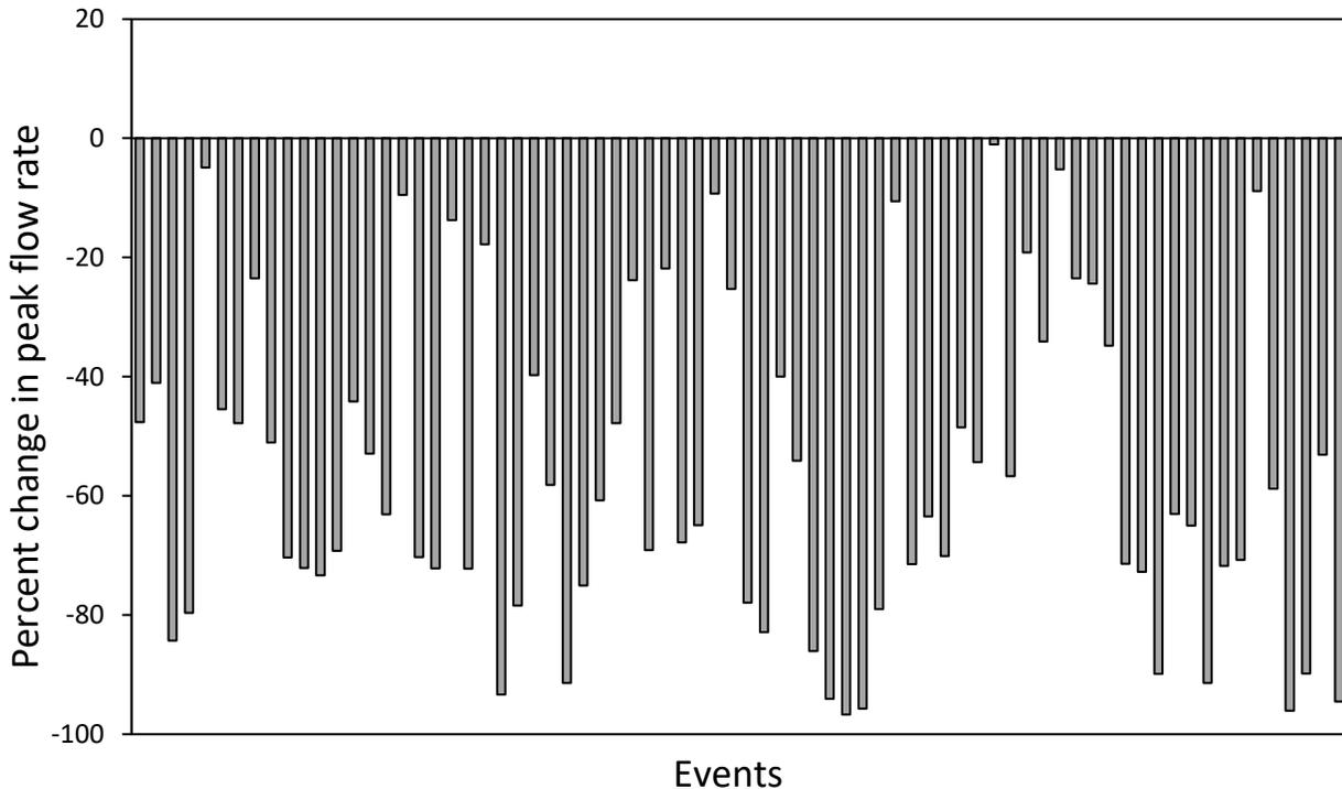
**Figure 12: Percentage change in peak flow rates between inflow and outflow runoff from a Water and Sediment Control Basin (June 2013 to September 2017).**
