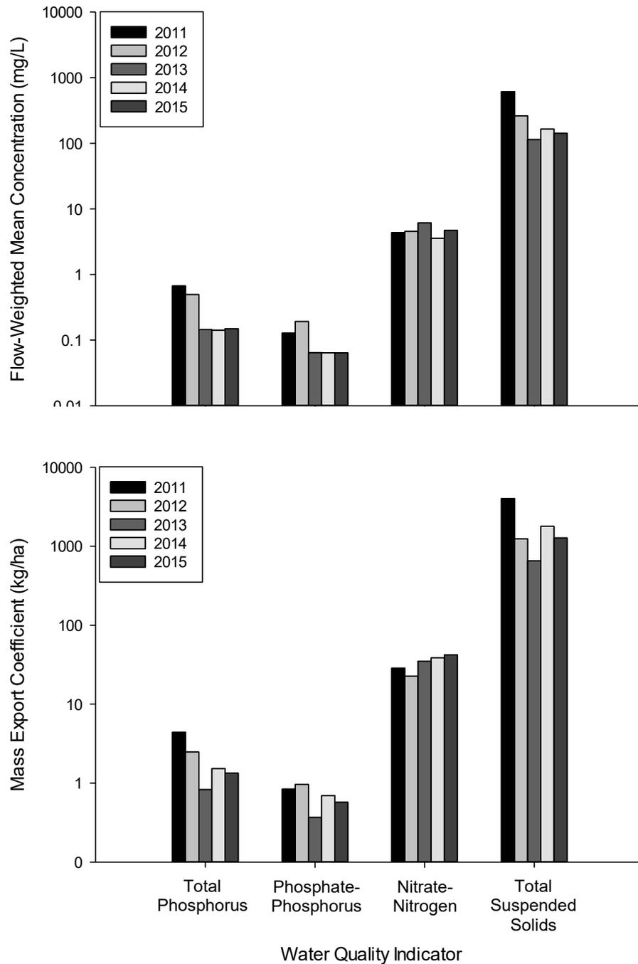
**Figure 3:** Annual flow-weighted mean concentrations and mass export coefficients in Gully Creek (October 1, 2010 – September 30, 2015). Notes: 1) Station GULGUL5 data were used to estimate mass export coefficients for the 2012-2015 water years. Station GULGUL2 data were used for the 2011 water year. The 2011 water year is October 1, 2010 to September 30, 2011. 2) A change of laboratory analysis method for total phosphorus occurred in 2013 at the Ministry of the Environment and Climate Change.
