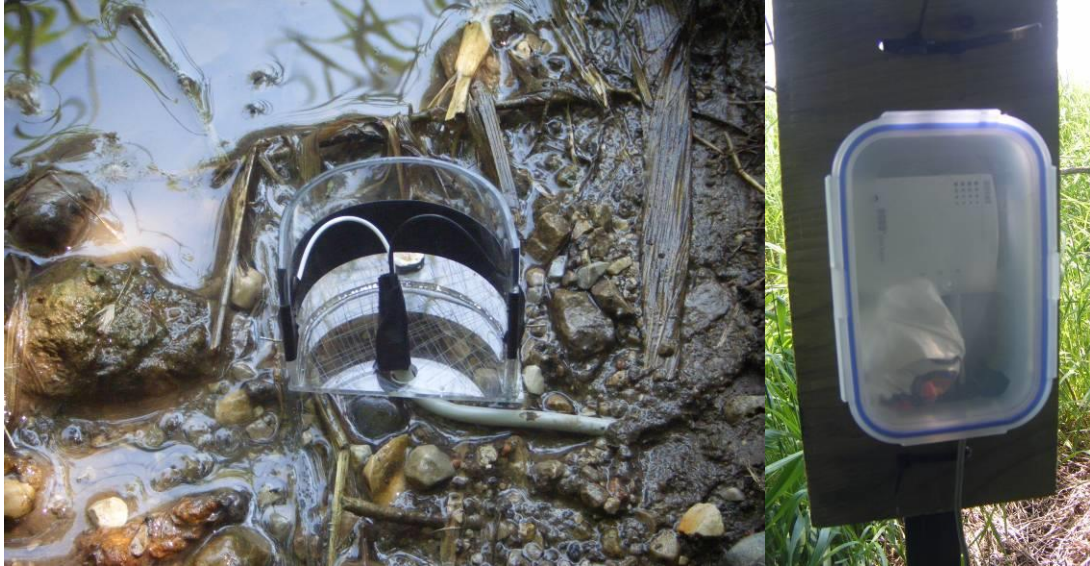
Plate 6.2: Flow sensor at the G11 property in the Gully Creek watershed.
