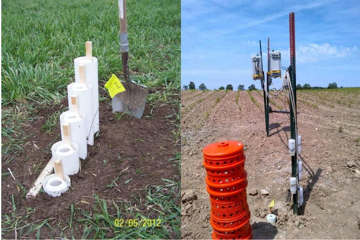
Plate 5.1: Water samplers installed at the G4 property in the Gully Creek watershed to monitor the Water and Sediment Control Basin inflow (left) and hickenbottom (right).
