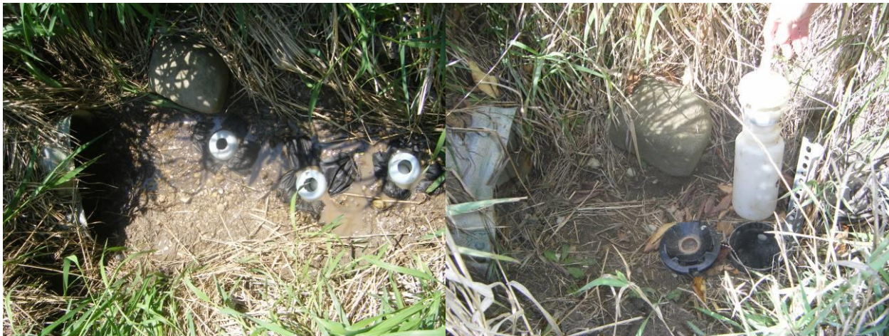
Plate 6.1: Two types of embedded water quality samplers at the G11 property in the Gully Creek watershed.
