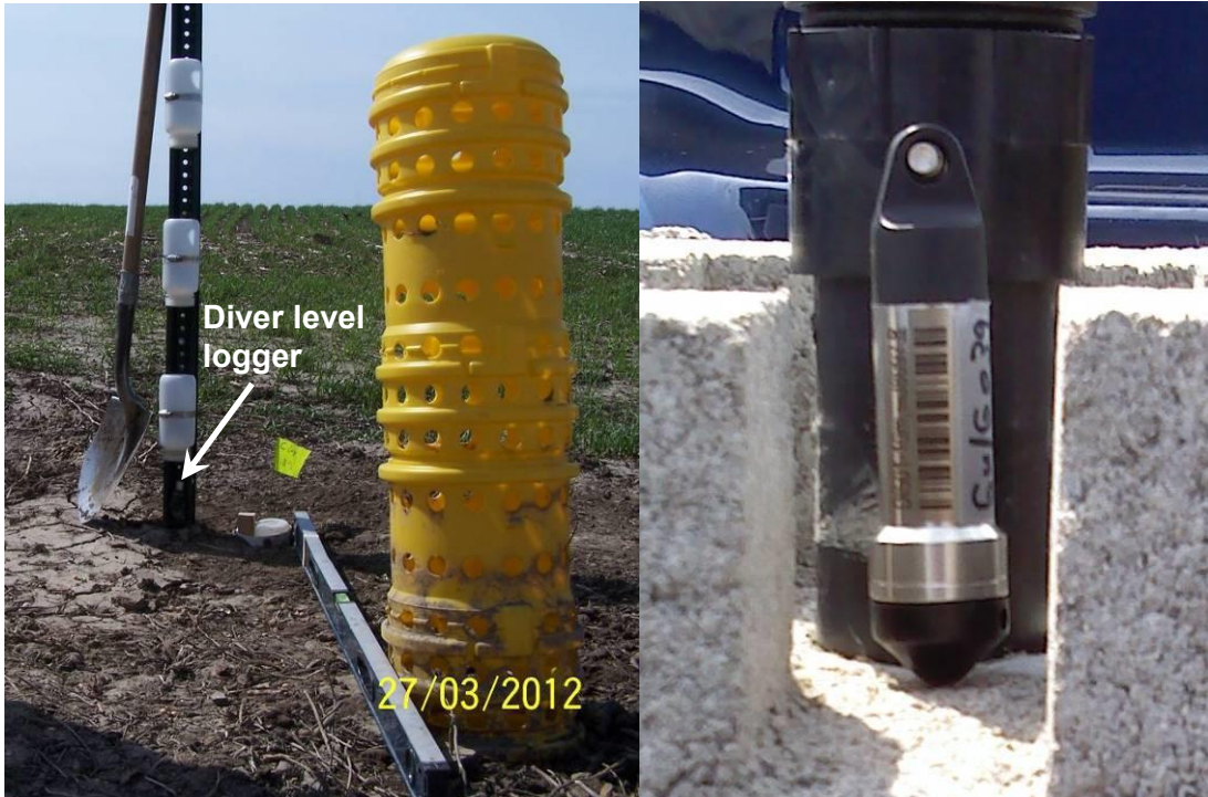
Plate 5.2: Diver® level logger installed at the G4 property in the Gully Creek watershed to monitor the water level in the Water and Sediment Control Basin ponding area.
