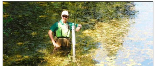
Ross Wilson, Water and Soils Resources Coordinator, installs staff gauge in the Old Ausable Channel.
