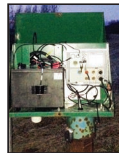
New data logging units that support satellite telemetry will be installed at eight sites across the watershed. ABCA and MOECC staff selected the sites in autumn of 2014.
