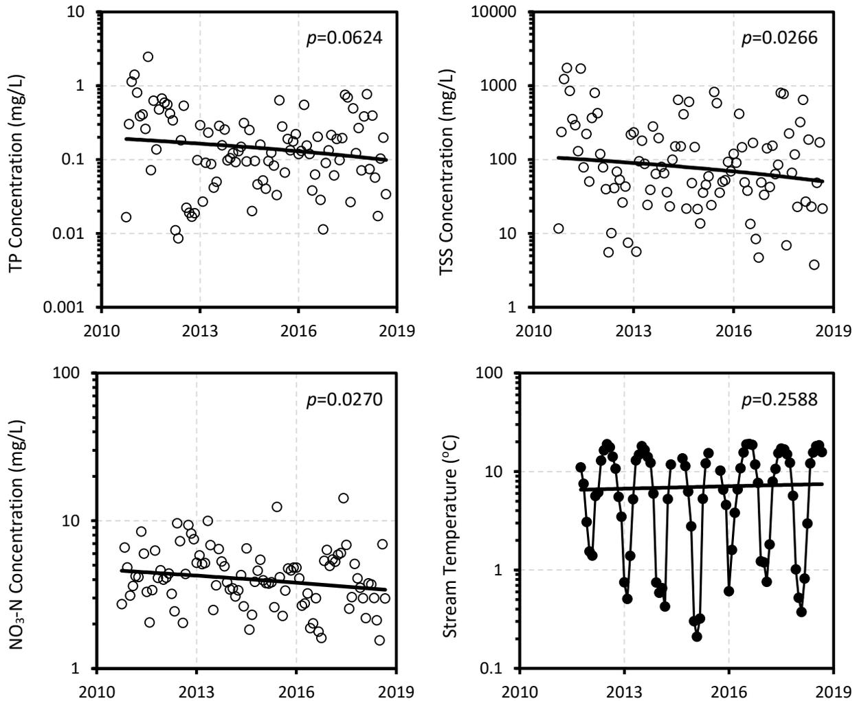
**Figure 6: An example of water quality trends in monthly flow-weighted mean concentrations and stream temperatures for Gully Creek (October 2010 to September 2018). Note: A change of laboratory analysis method for total phosphorus occurred in November 2012 at the Ministry of the Environment and Climate Change.**
