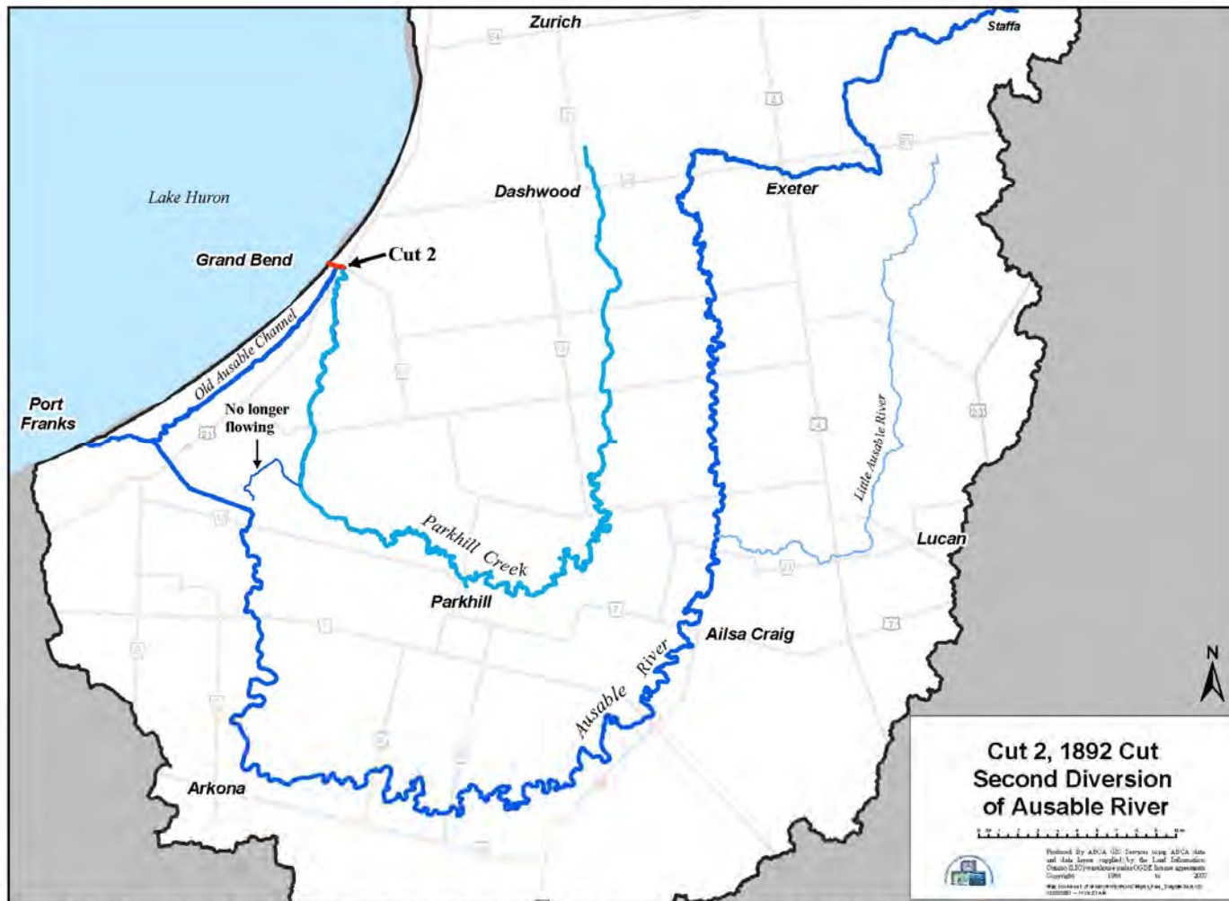
Figure 4: Configuration of the Ausable River and Parkhill Creek after a second diversion cut in 1892, which resulted in a harbor in Grand Bend
