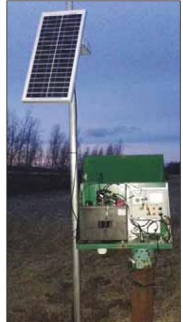
The Trick's Creek Overburden well was upgraded in 2013 with GOES satellite telemetry. This upgrade will provide near-real-time monitoring and, in addition to PGMN, will support Ontario Low Water Response. The Province of Ontario selected this site for that purpose.
