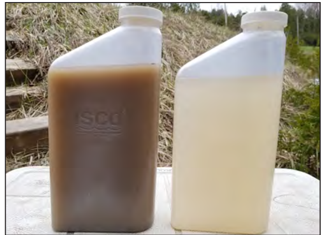
High sediment levels (bottle at left) can be associated with elevated phosphorus concentrations.
