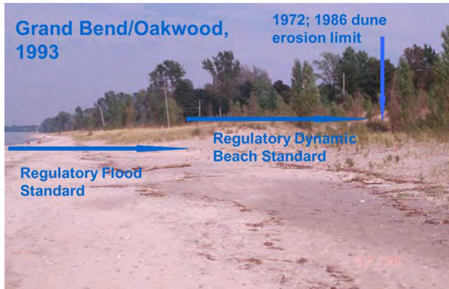
Figure 5.13: The test site at Oakwood used to determine the limit of wave erosion during major storms associated with periods of high lake level. Measurements here show that the maximum erosion is accommodated within a 30 m distance landward of the Regulatory Flood Standard. There is no long-term recession at this site.
