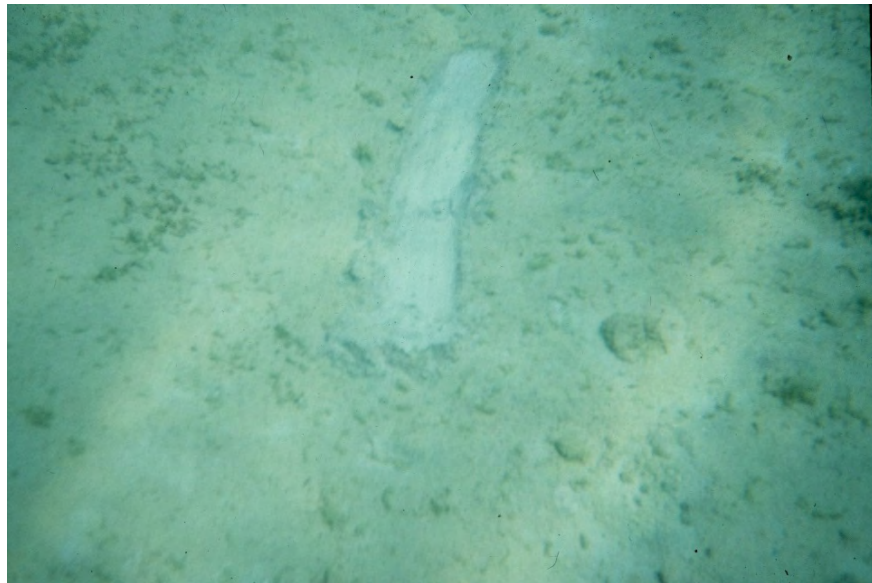
Figure 10: Underwater photo of till surface showing removal of a thin surface layer of weathered silt and clay by the finger of a wetsuit glove.
