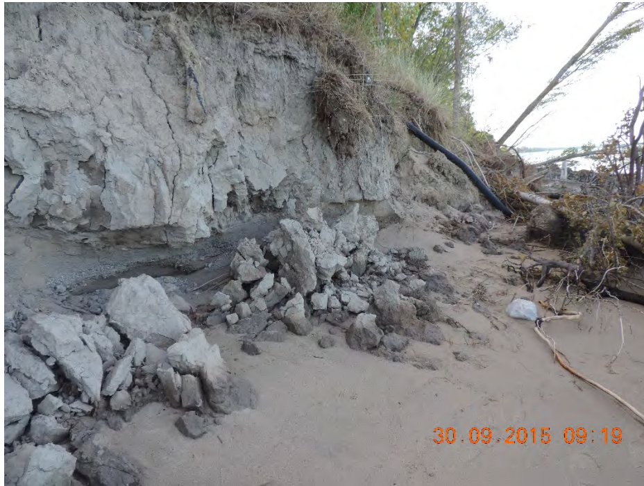
Figure 5: Desiccation cracks formed in a layer of weathered till leading to slumping of isolated blocks, ABCA shoreline
