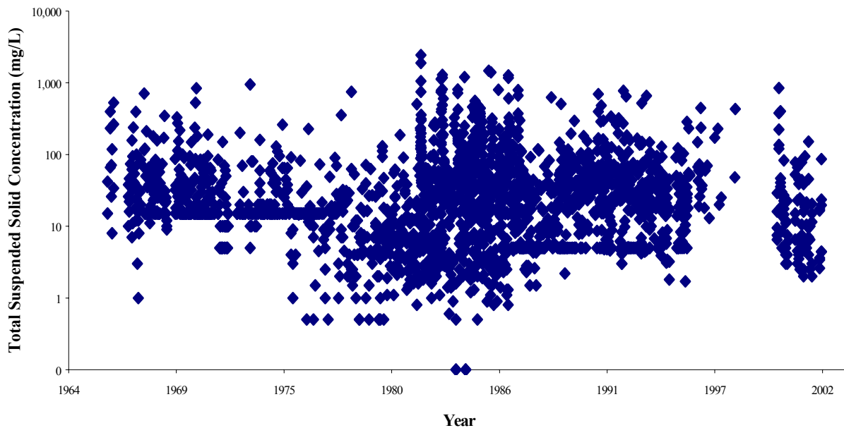
Figure 3.6: Total suspended solid concentrations (mg/L) at seven Provincial Water Quality Monitoring Network (PWQMN) stations in the Ausable River (n = 2336). For collection time periods at specific stations sites refer to Veliz (2003).
