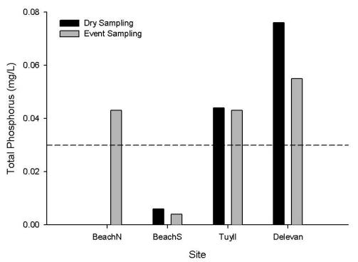
**Figure 3.** Dry (n=5) and event (n=5) sampling geometric mean total phosphorus concentrations in mg/L at four stormwater monitoring sites draining into Lake Huron along the shoreline of Bayfield, Ontario in 2014. Dashed line indicates Provincial Water Quality Objective of 0.030 mg/L.
